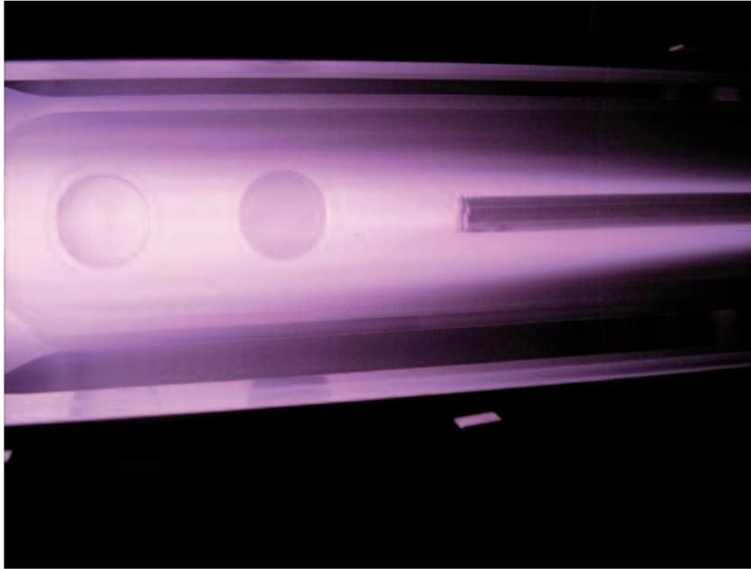
Fig. 4. Schematic of the MAGPIE device and a photo of the plasma interacting with a target.
